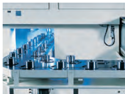
Automation for stand-alone machines: transport the workpieces to the pick-up position and remove the machined components
