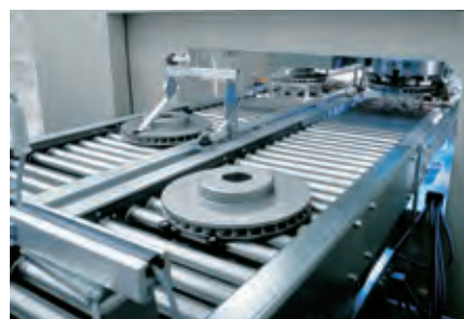
Twin-track loading for a quicker workpiece change
