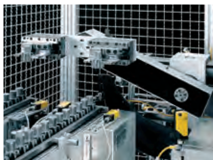
The twin-gripper collects a raw part from each feeder band and places them on the conveyor belt
