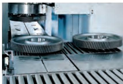
The workpieces are transported to the pick-up station and inserted into the chuck jaws
