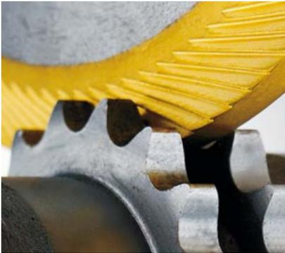
Deburring of a chain sprocket gears
