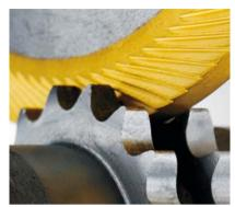
Deburring of a chain sprocket gears
