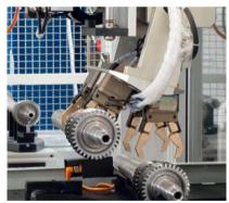
Gantry loader with double gripper
